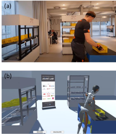
FIGURE 5: THE OPERATOR PERFORMS THE TASK (a) AND THE ERGONOMIST CAN ASSESS THE MANUAL OPERATION BY THE DIGITAL TWIN (b)
